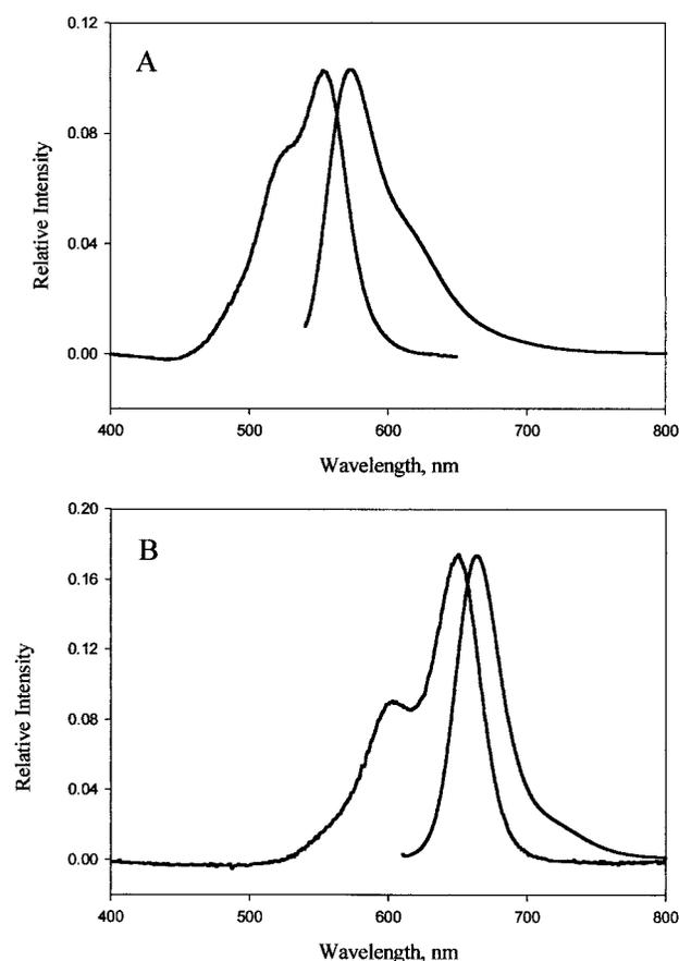
**Figure 2.** Normalized absorbance and fluorescence spectra of neo-Cy3-WASP (A) and neo-Cy5-WASP (B) conjugates in PBS (pH = 7.4), concentrations 1  $\mu\text{M}$ .
